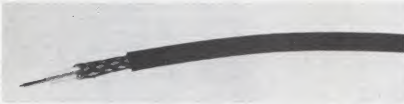
Photo 1: Coaxial cable consists of a central conductor, an outer conductive braid, and a protective coating. It is bulky and expensive, but it has good characteristics as a transmission line for data.
