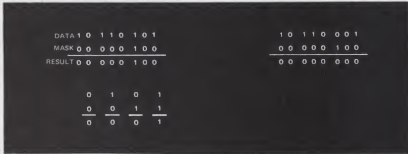
Figure 5: The AND function of Boolean logic is used to mask the current universe in order to select one position for testing each shot.
