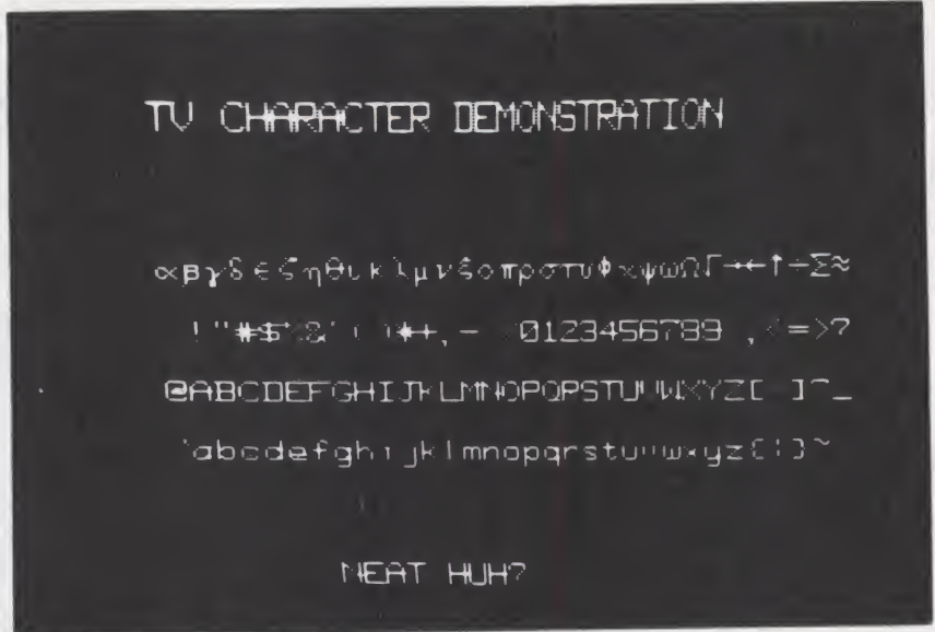
Photo 1: A test demonstration of Dr Suding's TV readout, shown in schematic form as figures 1 and 2. The test pattern consists of the four lines in the center which cycle through the possible binary combinations of characters. The differences in line width between the top line and the other lines are caused by non-linearities in the monitor used for this photograph.
