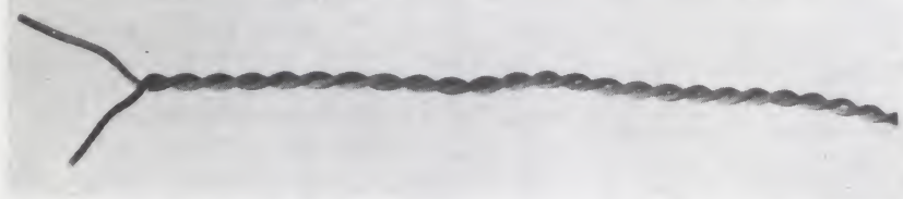
Photo 3: Twisted pair cable is the only good data transmission line which can be easily fabricated at home. Here is an example made using an electric drill to do the twisting.
