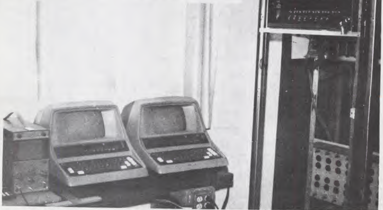
Photo 1: The author's computer setup includes the two CRT terminals shown on the table, plus a rack cabinet presently containing his central processor.
