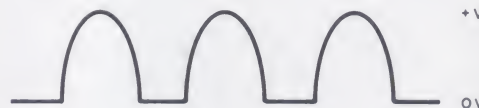
Figure 8: Voiced Sounds from the Glottis. Sounds which have definite pitch are called voiced sounds. In the natural larynx, these sounds are generated by the vocal chords and drive the vocal tract at the glottis. In an electronic analog, the voiced sounds can be generated by a programmable counter (to set the frequency) which in turn creates a sine wave of the same frequency. A rectified sine wave is a good source for the glottal pulses used in the electronic model of a larynx used in the author's approach to speech generation.
