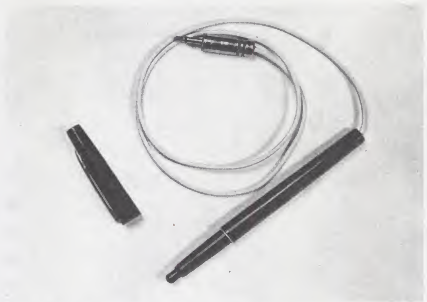
Photo 4: This shows a pen based on the TI type L-63 photocell, built using a marking pen case.
