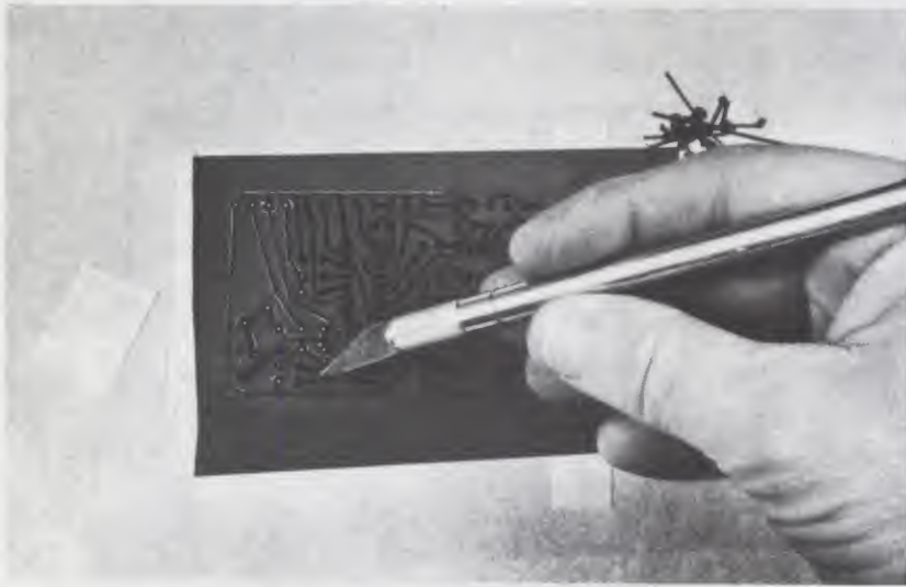
Photo 4: The "Cut-N-Peel" Method. A sheet of red mylar film on clear acetate backing is placed over the pattern to be copied. The negative is made by carefully tracing the pattern with a razor or sharp knife, then removing the red film wherever component pads and connections are to be made. (A trade name for the film used in this method is "Rbylith.") The negative is then transferred to sensitized copper and etched.
