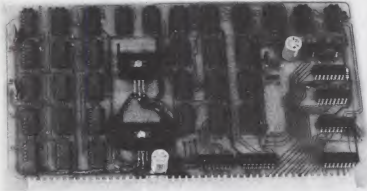
The memory board, shown here with a full 4096 word complement of 2102 memory chips, is one of the more important elements of the system. The black chips at the right edge of the photo are interface devices and address decoding. The two voltage regulators on the board are in the center. The remaining integrated circuits are 32 chips of 1 K by 1 bit memory.
