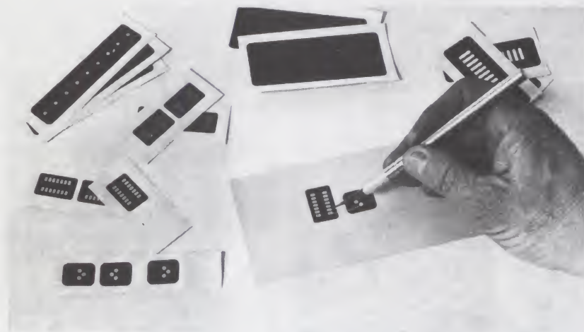
Photo 5: The Bishop Graphics "B' Neg" Method. In this method, a negative is made directly, using self adhesive black patterns on a mylar backing. The connections between patterns are made by cutting away the black layer with a sharp knife as in the "Cut-N-Peel" method.
