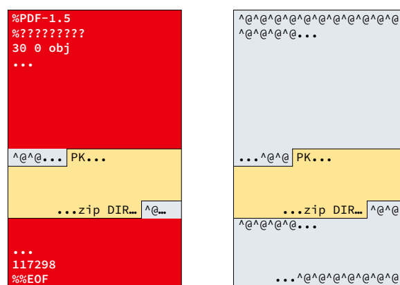
Figure 2: Padding the zip with incompressible bags of null characters solves the issue illustrated in Figure 1 by ensuring that the detached zip has the same offsets as the polyglot.
